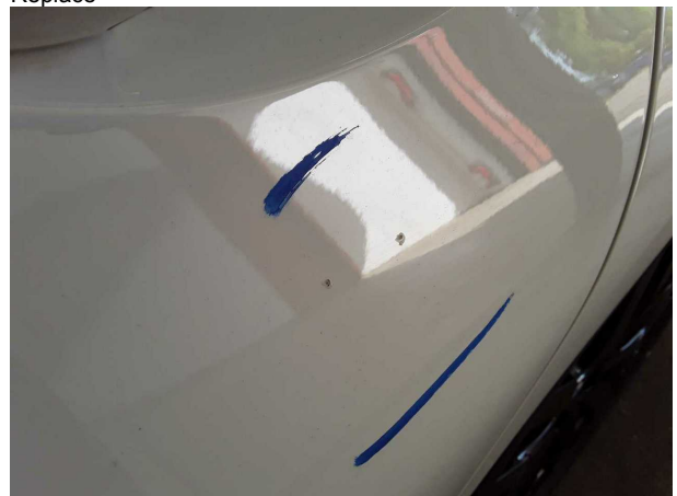
Damage #4: Door - rear left side: Door - Scratched - Repair a... paint
