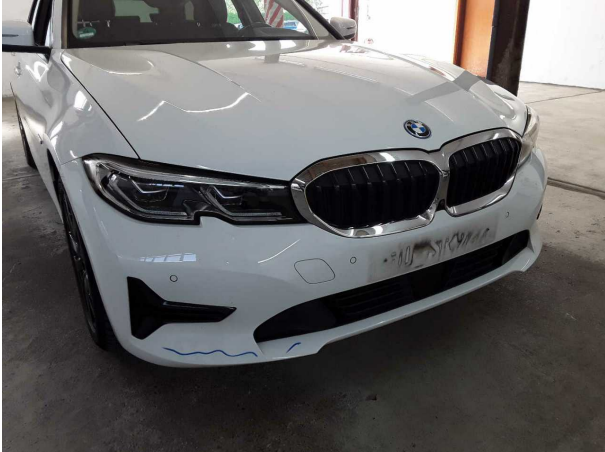
Damage #2: Front bumper: Front bumper - Scratched - Smart repair
