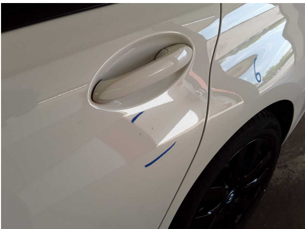
Damage #4: Door - rear left side: Door - Scratched - Repair and paint
