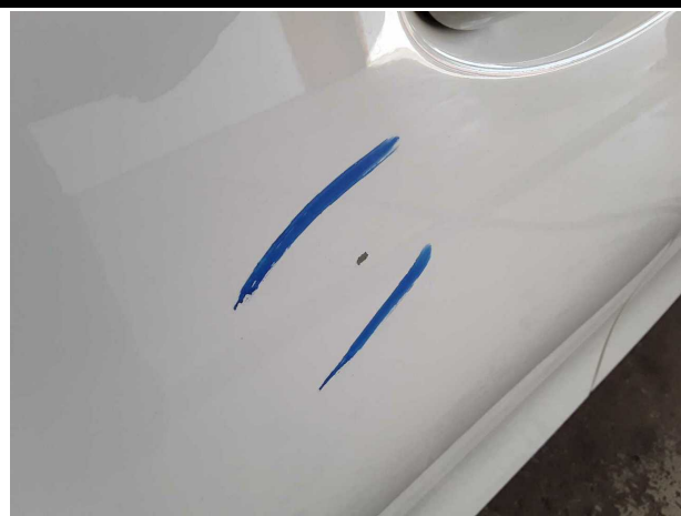
Damage #5: Door - front left side: Door - Scratched - Repair and paint
