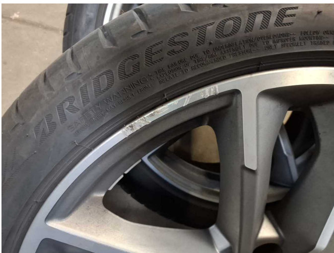
Damage 8: Wheel / tyres: Alloy rim - rear right side - Scratched - Loss in value
