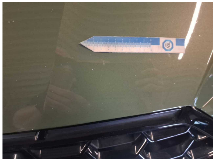
Damage 9: Bonnet: Bonnet - Stone chips - Paint
