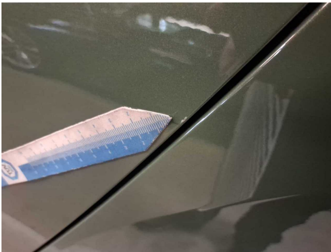
Damage 4: Door - rear left side: Door - Scratched - Smart repair
