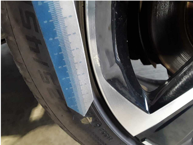
Damage 1: Wheel / tyres: Alloy rim - rear left side - Corrosion - Loss in value
