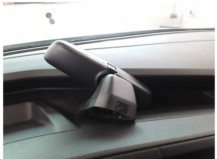
Damage 5: Instrument panel: Interior mirror - Damaged - Replace
