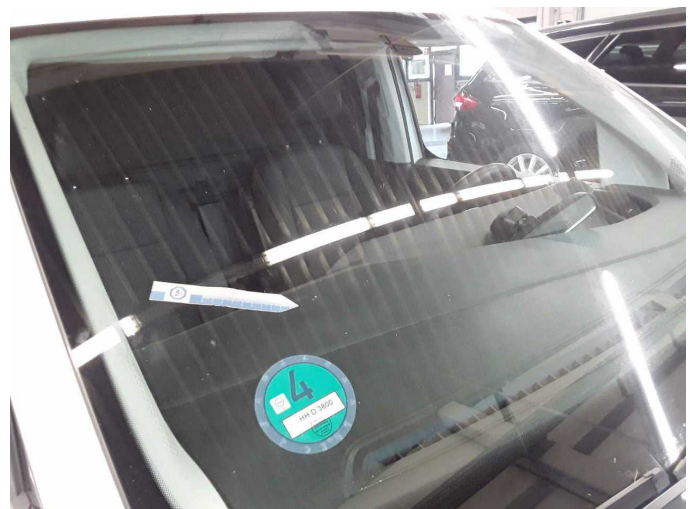
Damage 8: Vehicle glazing: Windscreen (Vermehrte steinschläge) - Stone chips - Replace
