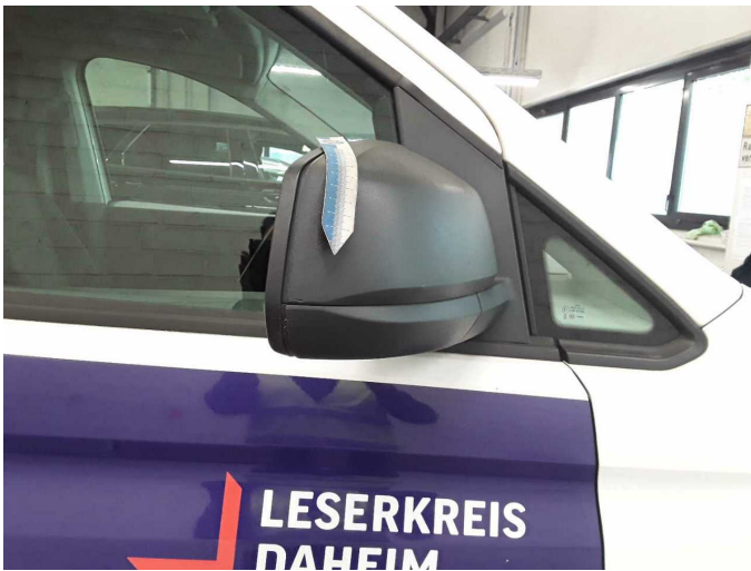
Damage 2: Wing mirror - right side: Cap - Scratched - Smart repair
