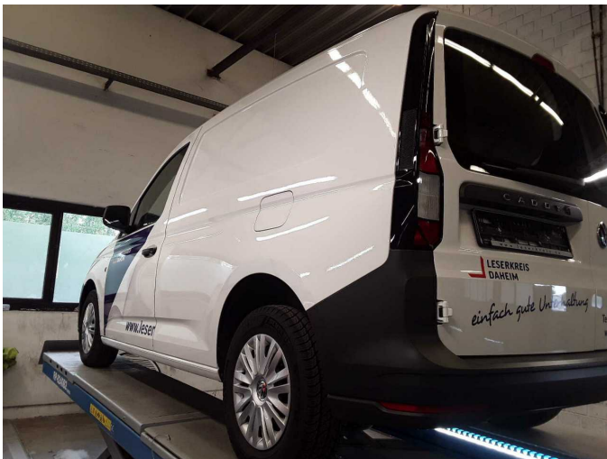
Damage 6: Body: Body - Glued / labelled - De-glue / neutralise
