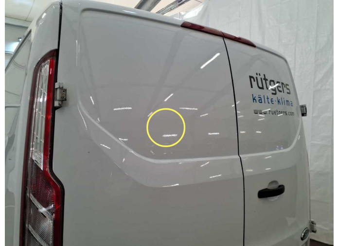
Damage 5: Boot lid / rear door: Rear door - left side - dent(s) - Smooth repair work
