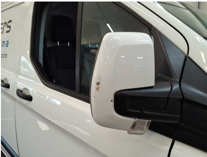
Damage 8: Wing mirror - right side: Cap - Scratch(es) - Paint
