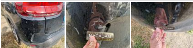
Bumper R, Deformed / Strained, Replace and paint
