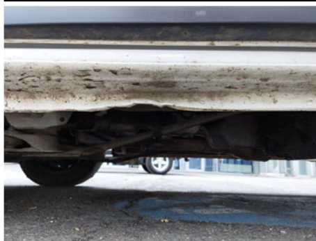
Schweller / Links / Delle
