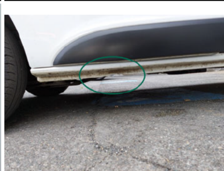
Schweller / Links / Delle
