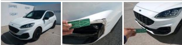
Bumper moulding FL, Scratch(es), Repair and paint (complete)
