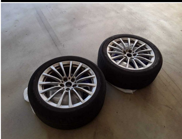
Damage #7: 2nd wheel set: 2 tyres - Porous / cracked - Replace
