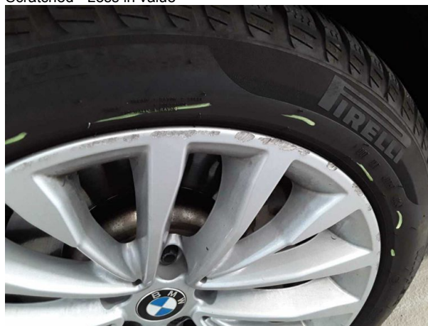
Damage #5: Wheel / tyres: Alloy rim - front left side - Scratched - Loss in value
