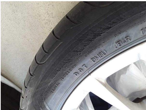
Damage #7: 2nd wheel set: 2 tyres - Porous / cracked - Replace
