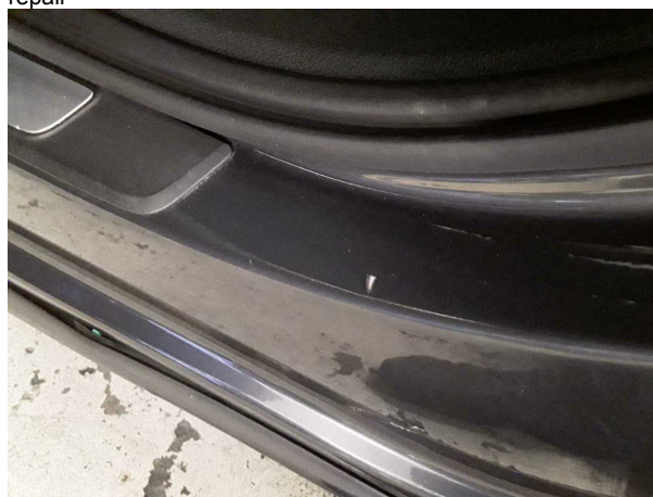
Damage #5: Side panel - rear left side: Sill - Dent / paintcoat damage - Smart repair
