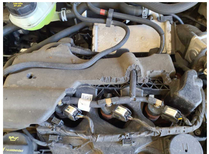
Damage 2: Engine: Engine cover - Damage caused by marten / rodent - Replace
