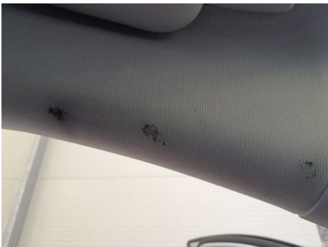
Damage 7: Trim / covers: Roof lining - Holes - Loss in value
