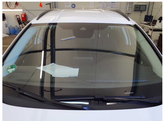
Damage 8: Vehicle glazing: Windscreen with lane departure assistant - Broken / torn - Replace
