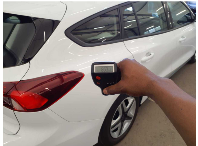
Repainting 1: Side panel - rear right side
