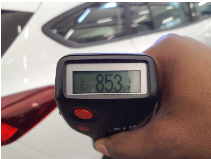
Repainting 1: Side panel - rear right side
