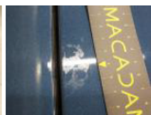
Bumper F, Scratch(es), Spot repair
