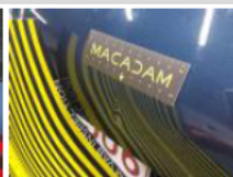
Tailgate / Boot, Dent(s), Paintless dent repair
