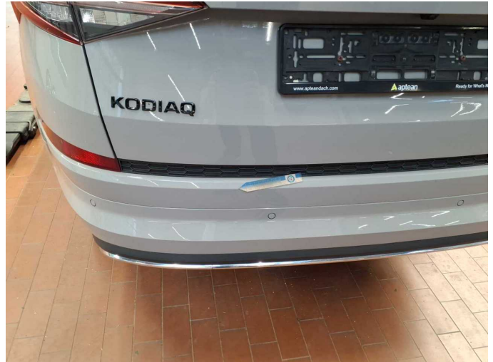
Damage 2: Rear bumper: Rear bumper - Scratch(es) - Paint
