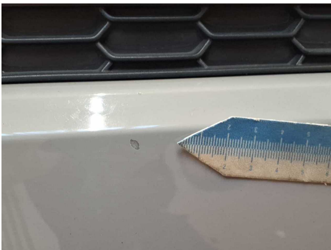
Damage 2: Rear bumper: Rear bumper - Scratch(es) - Paint
