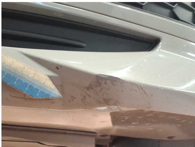
Damage 5: Front bumper: Spoiler - Scratched - Replace
