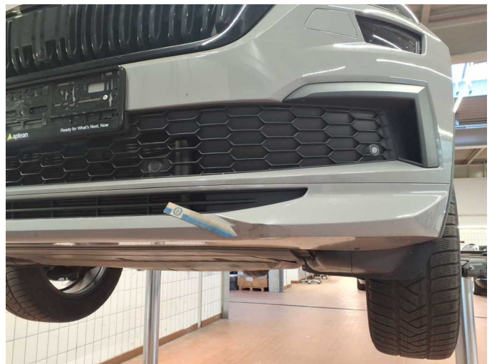
Damage 5: Front bumper: Spoiler - Scratched - Replace
