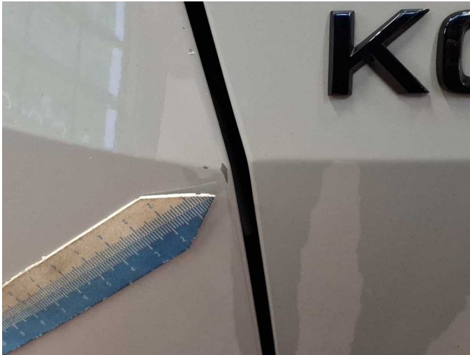
Damage 2: Rear bumper: Rear bumper - Scratch(es) - Paint
