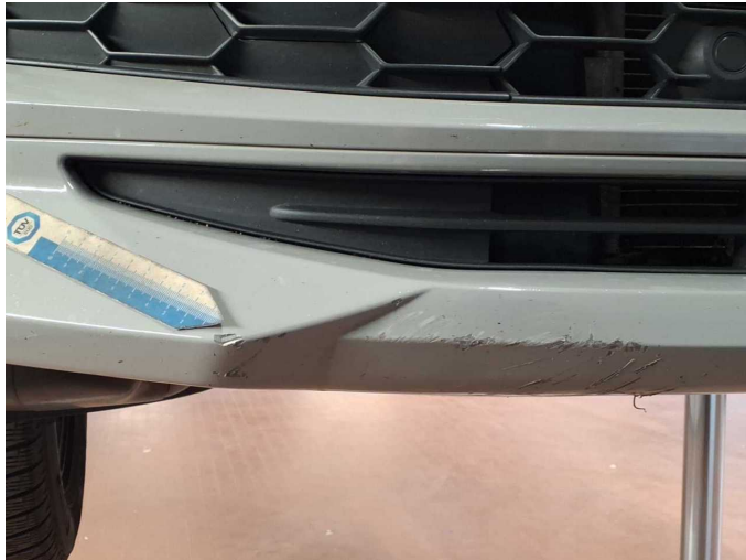
Damage 5: Front bumper: Spoiler - Scratched - Replace
