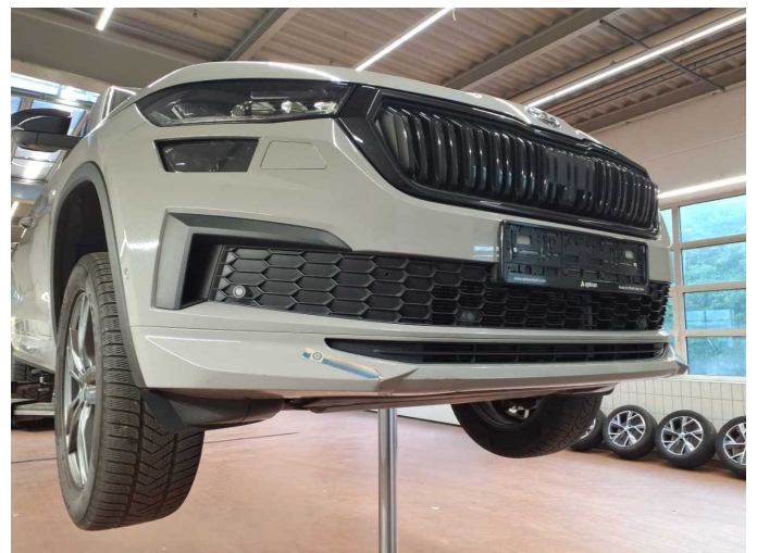
Damage 5: Front bumper: Spoiler - Scratched - Replace
