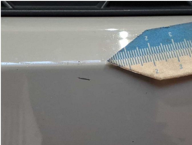
Damage 2: Rear bumper: Rear bumper - Scratch(es) - Paint
