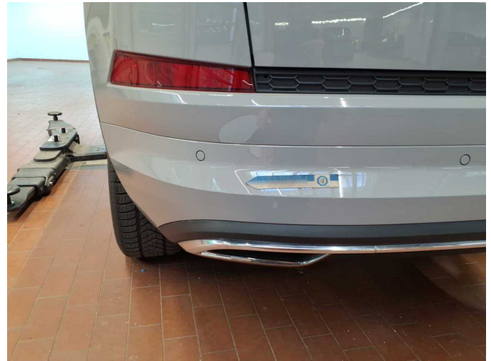
Damage 3: Rear bumper: Spoiler - Dent / paintcoat damage - Repair and paint
