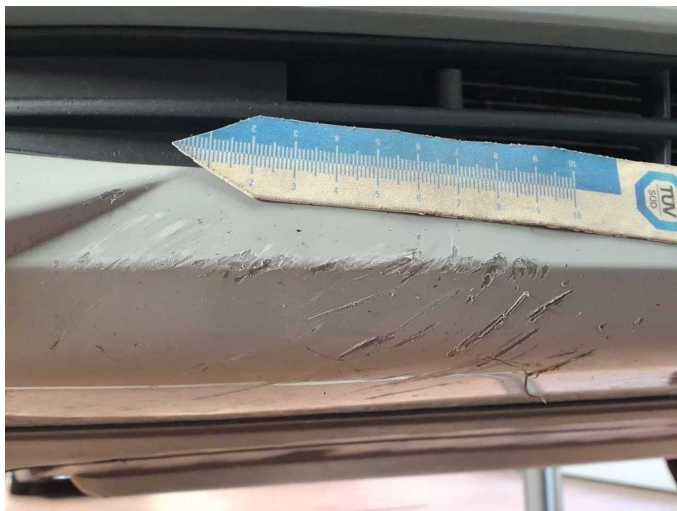
Damage 5: Front bumper: Spoiler - Scratched - Replace
