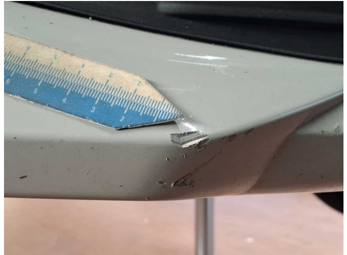
Damage 5: Front bumper: Spoiler - Scratched - Replace
