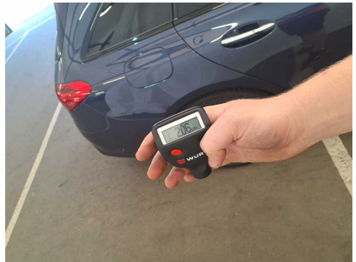
Repainting 1: Side panel - rear right side
