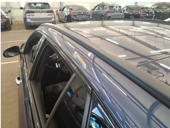
Damage 3: Roof: Roof rail - left side - dent(s) - Smooth repair work
