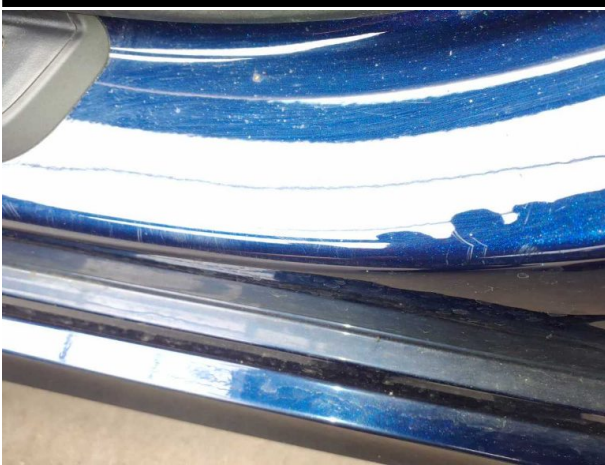
Damage #4: Sill - left side: Sill - Scratch(es) - Repair and paint
