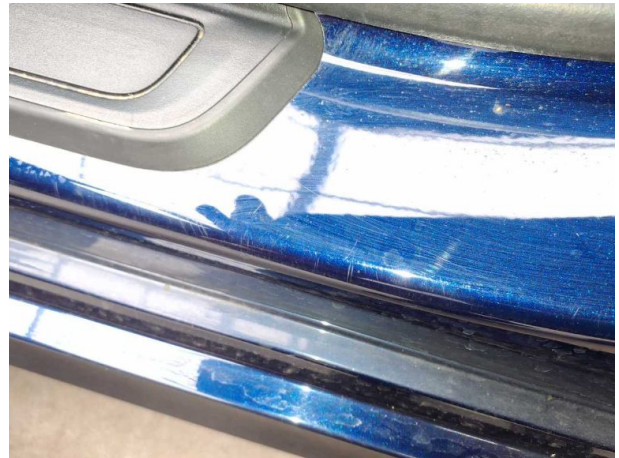
Damage #4: Sill - left side: Sill - Scratch(es) - Repair and paint
