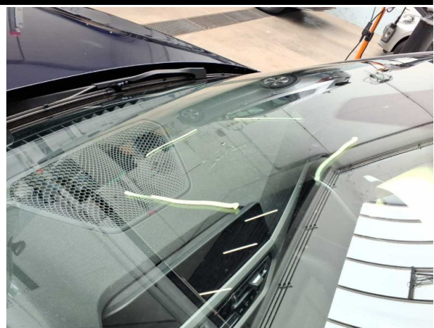
Damage #7: Vehicle glazing: Windscreen with lane departure assistant - Broken / torn - Replace
