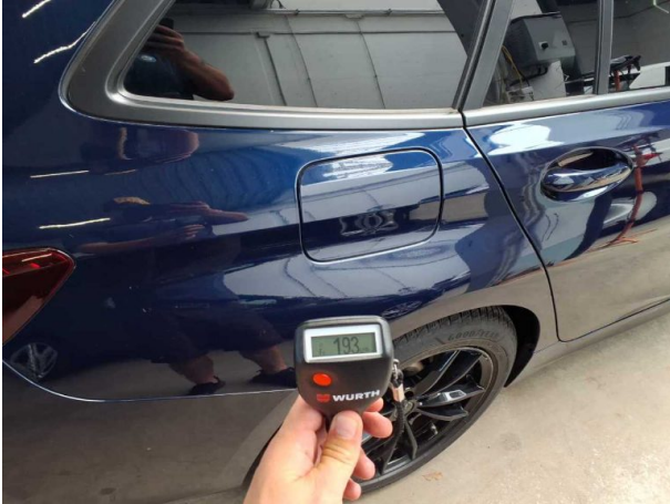
Repainting 1: Side panel - rear right side
