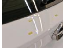
Tailgate / Boot, Dent(s), Repair and paint (complete)
