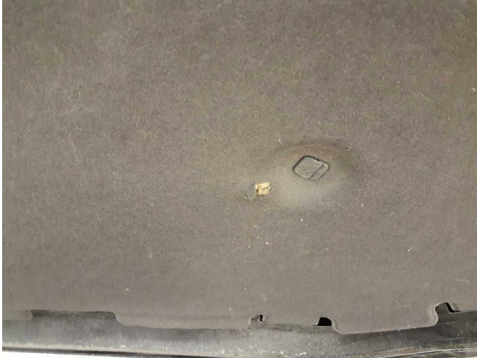
Damage 2: Bonnet: Insulation lining - Broken / torn - Replace
