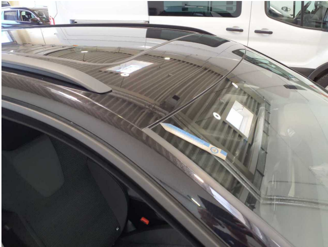
Damage 15: Roof: Roof - Scratch(es) - Repair and paint
