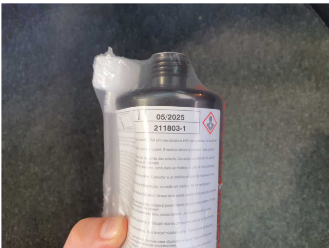
Damage 1: Equipment: Tirefit filler - Expired - Replace
