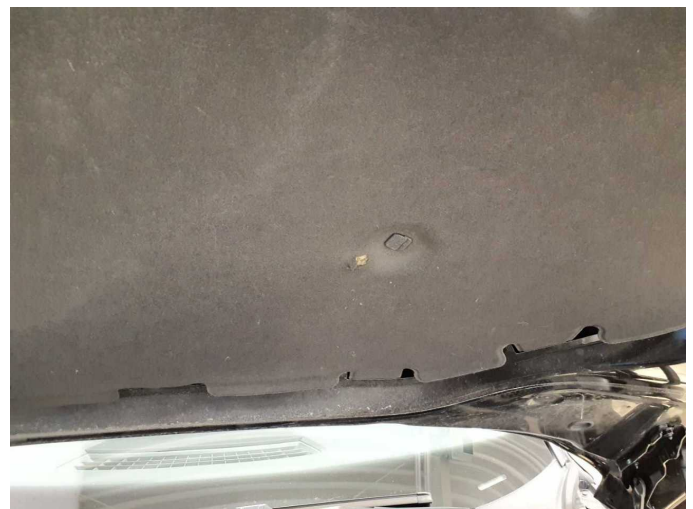
Damage 2: Bonnet: Insulation lining - Broken / torn - Replace
