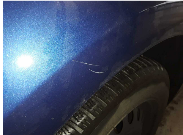
Damage #1: Mudguard - left side: Mudguard - left side - Scratched - Smart repair
