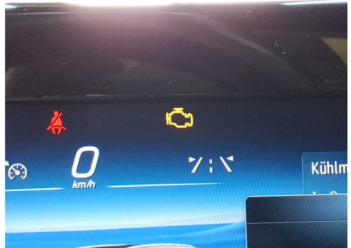
Damage 8: Instrument panel: Indicator light (Motorkontrolleuchte) - on - Perform
