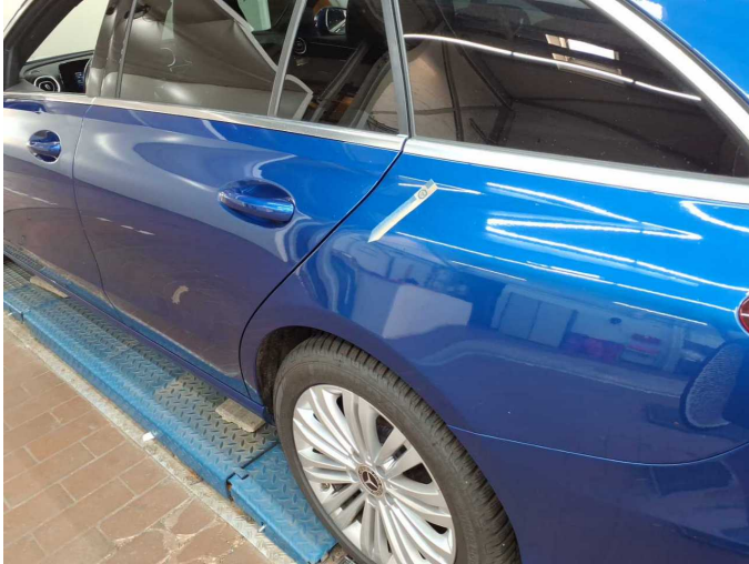
Damage 10: Side panel - rear left side: Side panel (Orangenhaut) - Unprofessionally repaired - Paint
