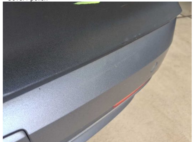
Damage #6: Rear bumper: Spoiler - Scratched - Loss in value
