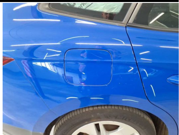
Damage #14: Side panel - rear right side: Side panel - Scratch(es) - Repair and paint
