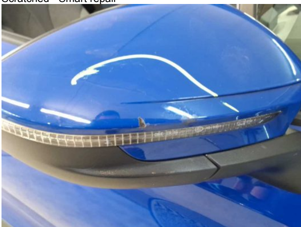
Damage #9: Wing mirror - right side: Cap - Scratched - Smart repair
