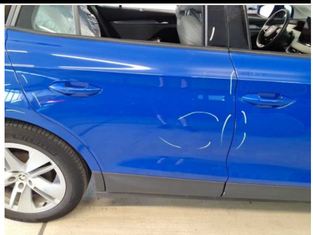
Damage #13: Door - rear right side: Door - Scratch(es) - Repair and paint
