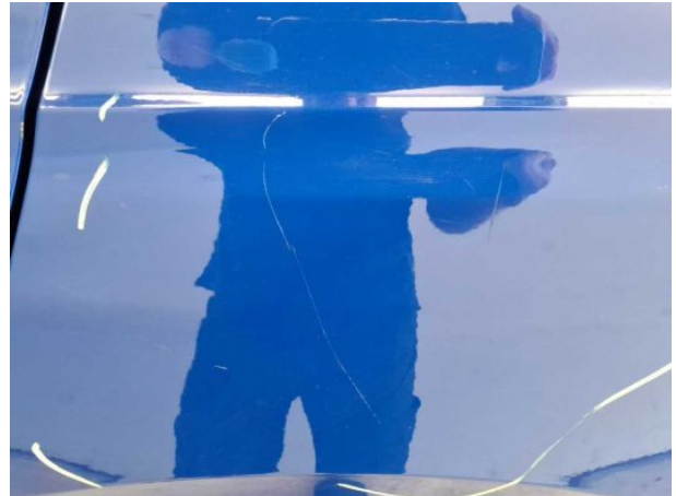
Damage #2: Side panel - rear left side: Side panel - Scratch(...) - Cover / polish
