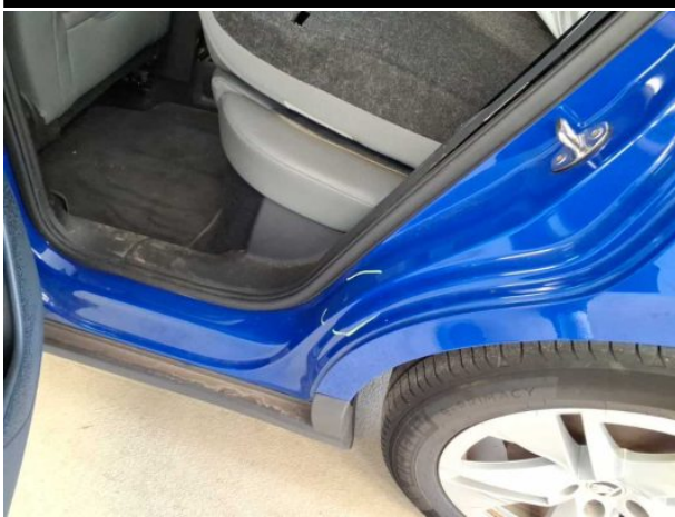
Damage #7: Side panel - rear left side: Sill - Dent / paintcoat damage - Smart repair
