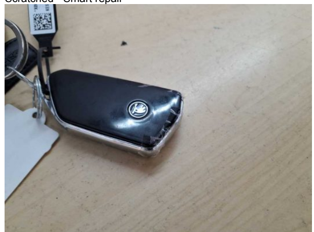
Damage #11: Equipment: Vehicle key with remote control - Damaged - Replace
