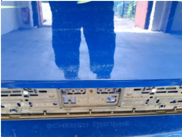
Damage #15: Boot lid / rear door: Boot lid - Scratched - Repair and paint
