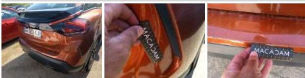
Bumper moulding R, Scratch(es), Replace
