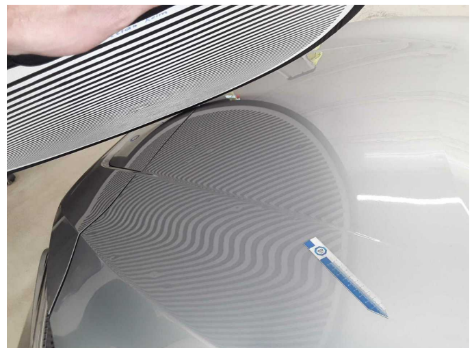
Damage 12: Body: Body (Hagelschaden) - dent(s) - Repair
