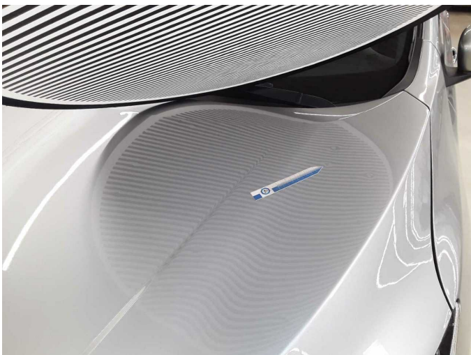
Damage 12: Body: Body (Hagelschaden) - dent(s) - Repair
