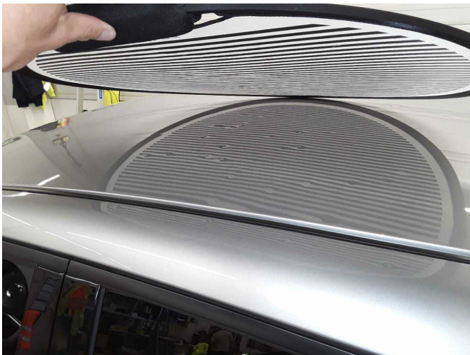
Damage 12: Body: Body (Hagelschaden) - dent(s) - Repair
