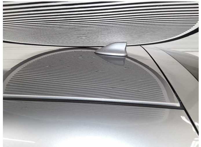
Damage 12: Body: Body (Hagelschaden) - dent(s) - Repair
