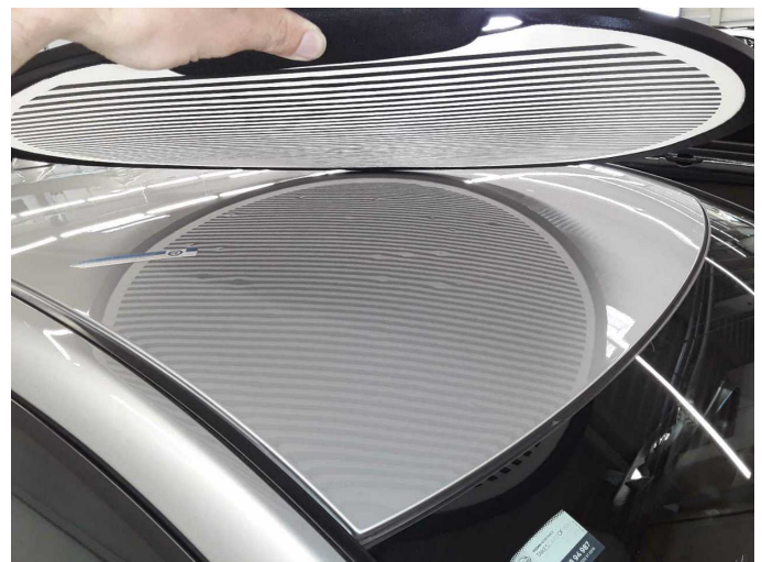
Damage 12: Body: Body (Hagelschaden) - dent(s) - Repair
