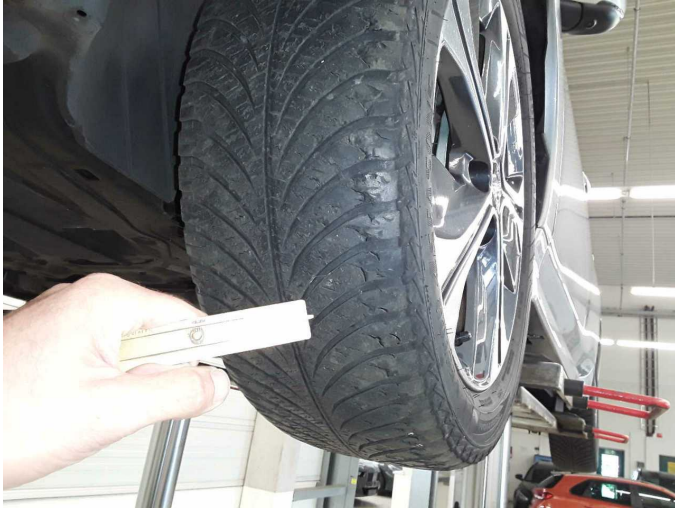
Damage 8: Wheel / tyres: Tyre - front - Does not meet the leasing specifications - Replace
