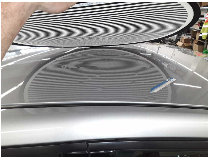
Damage 12: Body: Body (Hagelschaden) - dent(s) - Repair
