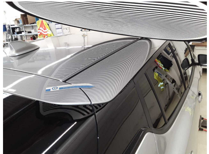
Damage 12: Body: Body (Hagelschaden) - dent(s) - Repair
