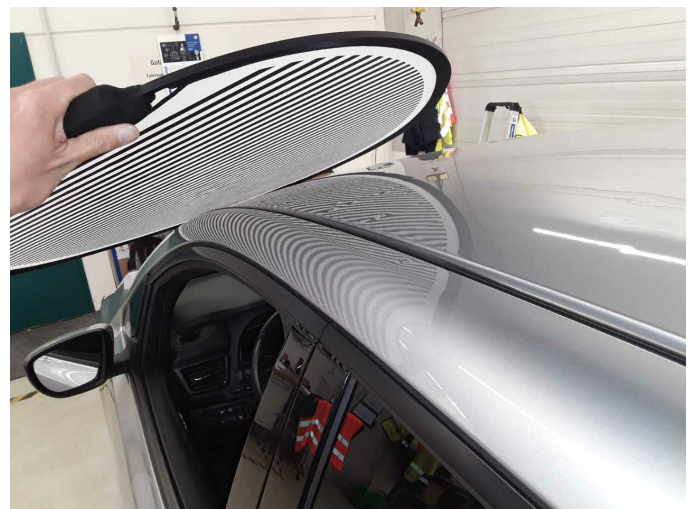
Damage 12: Body: Body (Hagelschaden) - dent(s) - Repair
