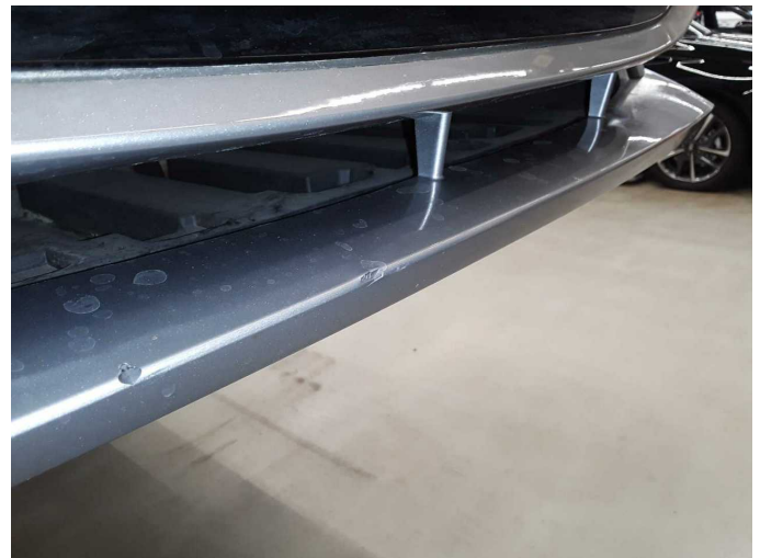
Damage 10: Front bumper: Front bumper - Scratched - Repair and paint
