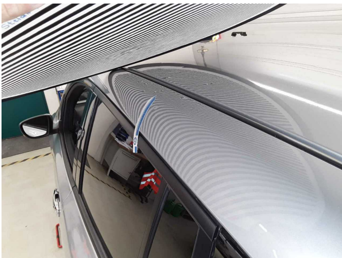
Damage 12: Body: Body (Hagelschaden) - dent(s) - Repair
