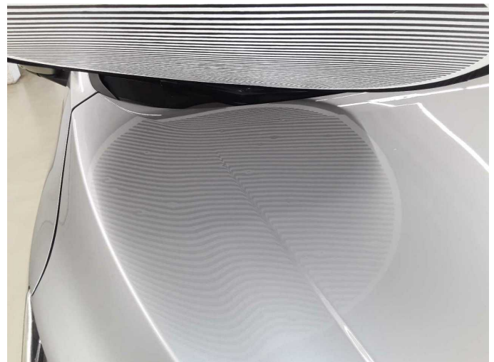
Damage 12: Body: Body (Hagelschaden) - dent(s) - Repair
