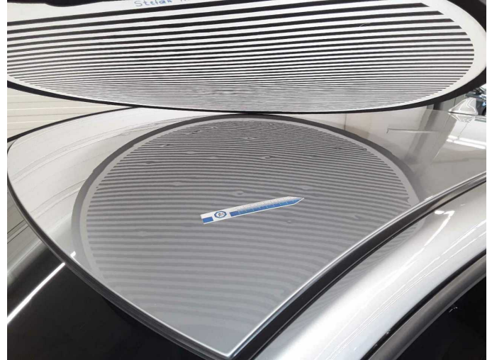
Damage 12: Body: Body (Hagelschaden) - dent(s) - Repair
