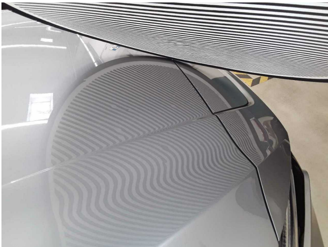
Damage 12: Body: Body (Hagelschaden) - dent(s) - Repair
