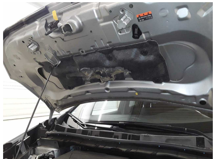
Damage 7: Bonnet: Insulation lining - Broken / torn - Replace
