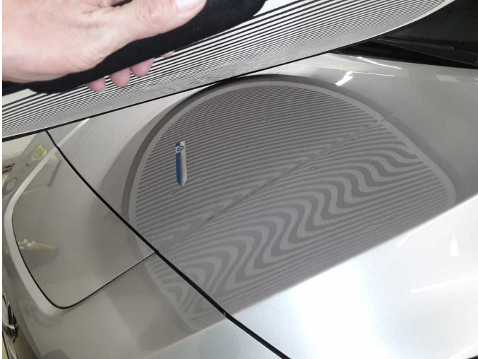
Damage 12: Body: Body (Hagelschaden) - dent(s) - Repair
