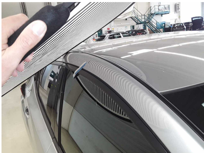
Damage 12: Body: Body (Hagelschaden) - dent(s) - Repair
