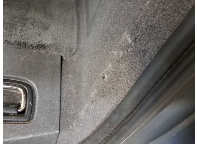
Damage 5: Side panel - rear right side: Interior trim (Stoff) - Broken / torn - Smart repair
