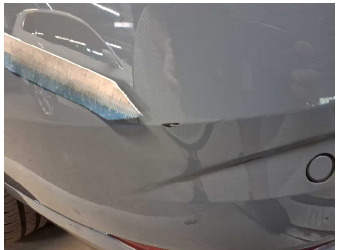
Damage 17: Rear bumper: Rear bumper - Scratched - Paint
