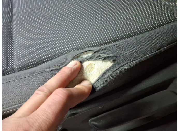
Damage 15: Seat - front: Seat cover - left side (+ Polster) - Broken / torn - Replace
