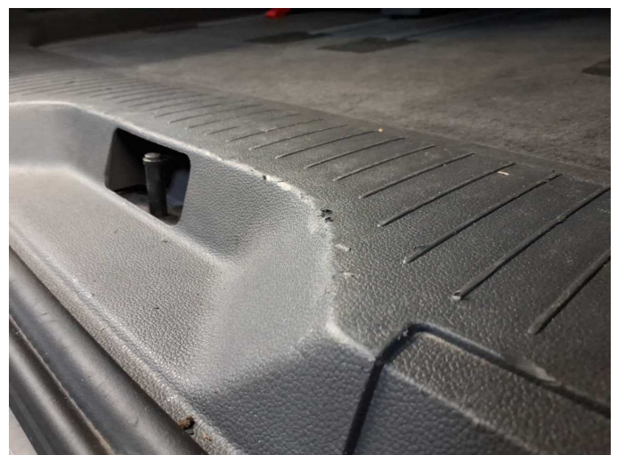
Damage 6: Trim / covers: Boot sill cover (Materialabtrag) - Scratched - Replace
