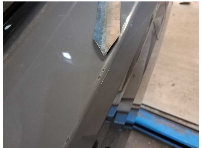
Damage 17: Rear bumper: Rear bumper - Scratched - Paint
