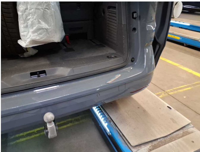
Damage 17: Rear bumper: Rear bumper - Scratched - Paint
