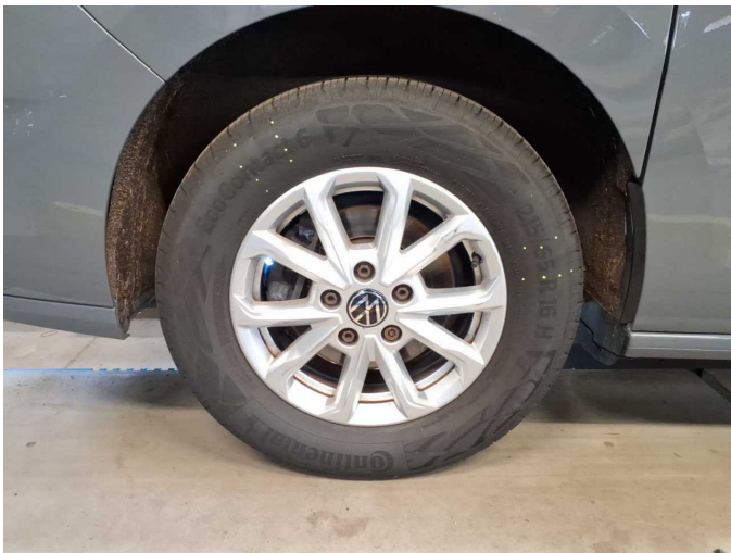
Damage 7: Wheel / tyres: Tyre - rear right side (nicht fahrbereit) - Deformed - Replace
