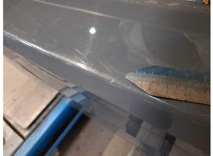
Damage 17: Rear bumper: Rear bumper - Scratched - Paint
