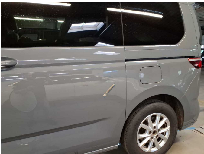
Damage 16: Sliding door - left side: Sliding door with glass panel - Scratch(es) - Paint
