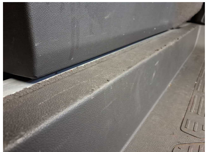
Damage 13: Trim / covers: Entrance sliding door - left side (Trittbrett links Materialabtrag) - Scratched - Replace
