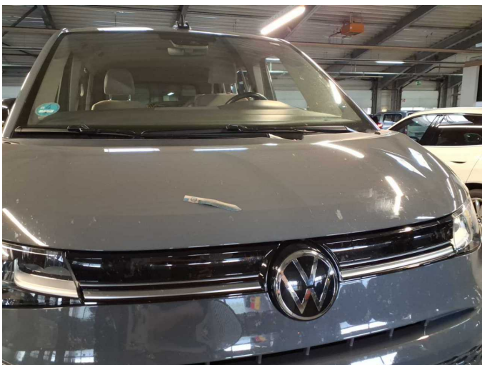
Damage 19: Bonnet: Bonnet - Dent / paintcoat damage - Repair and paint
