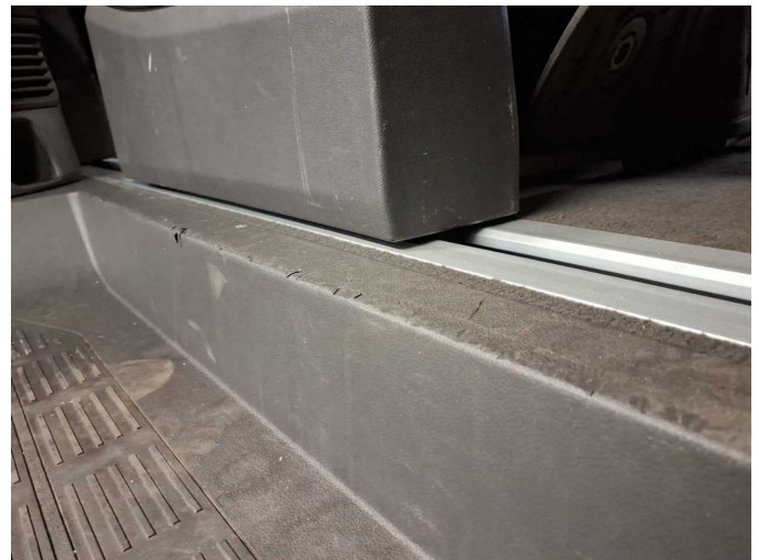
Damage 14: Trim / covers: Entrance sliding door - right side (Trittbrett rechts Materialabtrag) - Scratched - Replace
