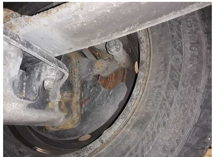
Damage 3: Braking system: Brake discs and pads - rear - Corrosion - Replace
