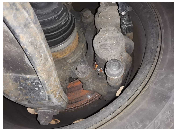
Damage 4: Braking system: Brake discs and brake pads - front - Corrosion - Replace
