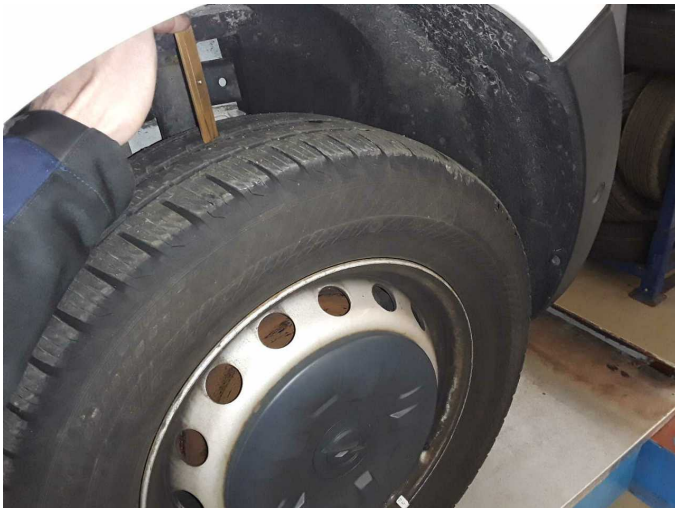
Damage 2: Wheel / tyres: Tyre - front - Does not meet the leasing specifications - Replace
