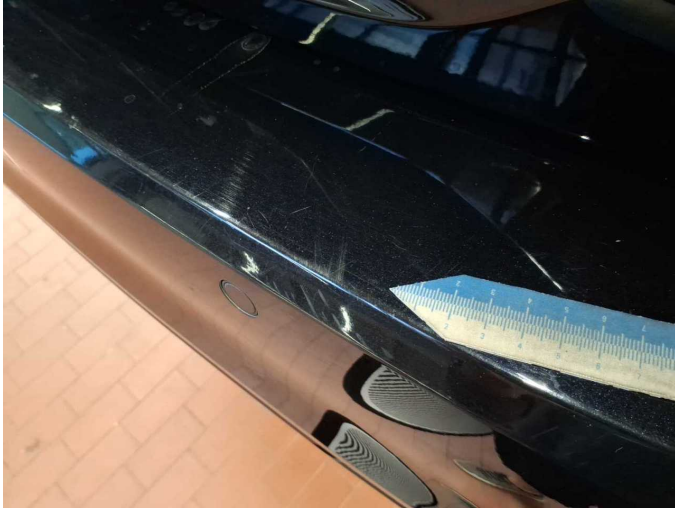
Damage 3: Rear bumper: Rear bumper - Scratch(es) - Paint
