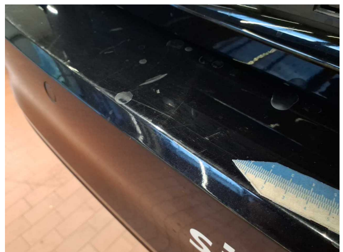
Damage 3: Rear bumper: Rear bumper - Scratch(es) - Paint
