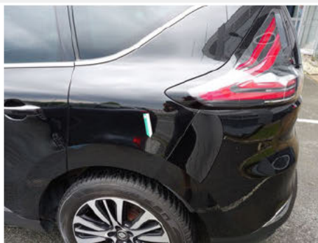
Kotflügel / Hinten Links / Delle
