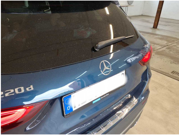
Damage 4: Boot lid / rear door: Boot lid - dent(s) - Repair and paint
