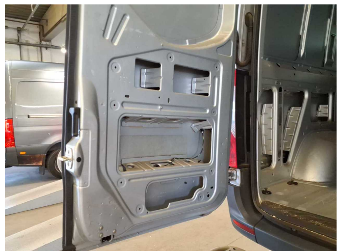
Damage 2: Trim / covers: Boot lid - interior trim (Links + Rechts) - Missing - Replace
