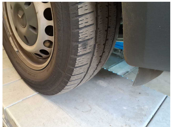
Damage 4: Wheel / tyres: Tyre - front (4mm) - Does not meet the leasing specifications - Replace
