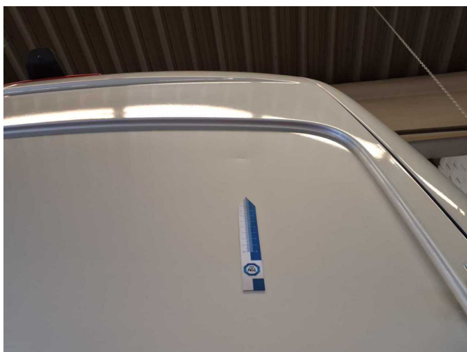
Damage 1: Boot lid / rear door: Rear door - right side - dent(s) - Smooth repair work
