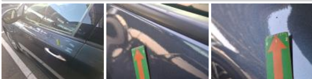
Door RL, Bad repair, Paint
