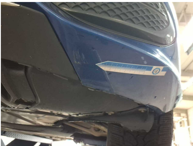
Damage 6: Front bumper: Front bumper - Scratch(es) - Paint
