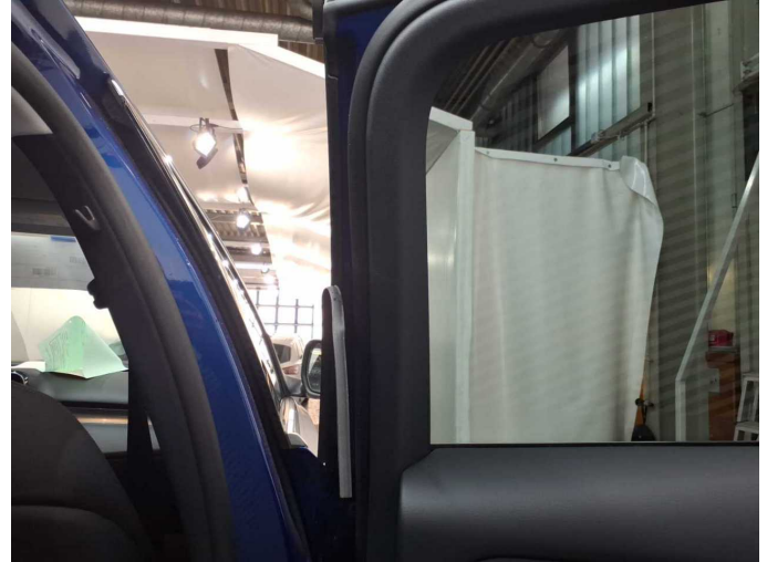
Damage 5: Door - rear right side: Window guide - Loose - Replace
