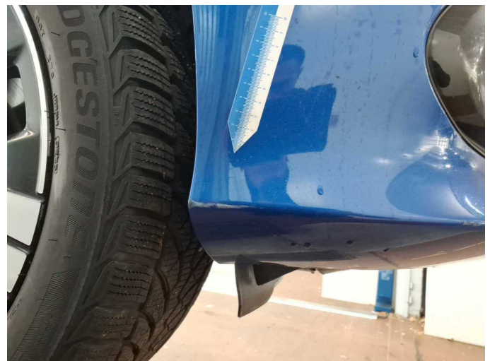
Damage 6: Front bumper: Front bumper - Scratch(es) - Paint
