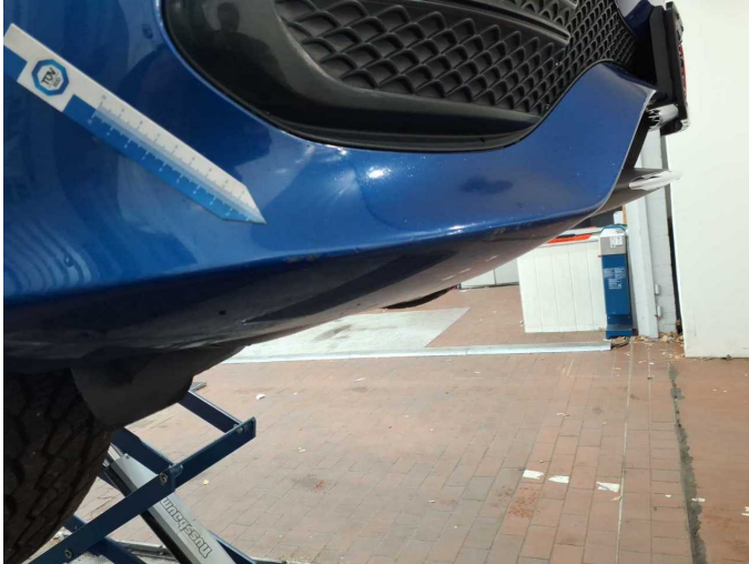
Damage 6: Front bumper: Front bumper - Scratch(es) - Paint
