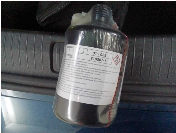
Damage 1: Equipment: Tirefit filler - Expired - Replace
