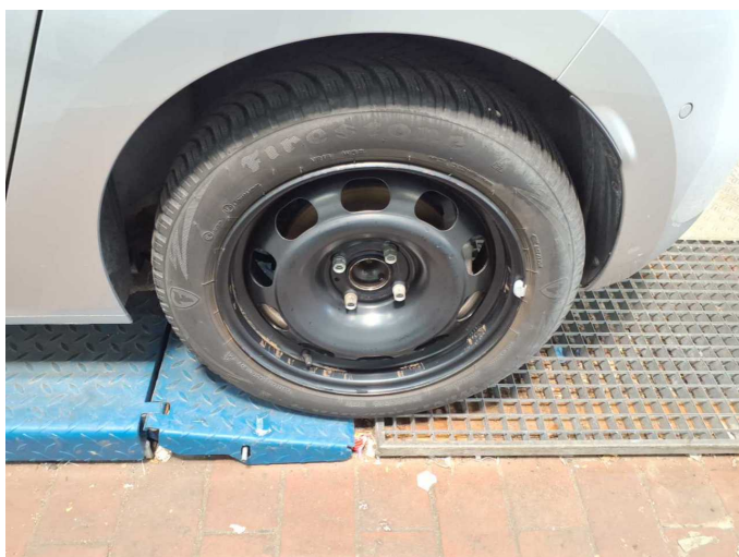
Missing part 1: Wheel / tyres: Wheel rim - rear left side (Radkappe fehlt) - Missing - Replace
