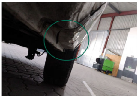
Schweller / Hinten Links / Delle
