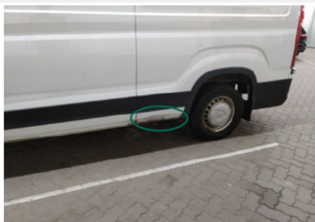
Schweller / Hinten Links / Delle
