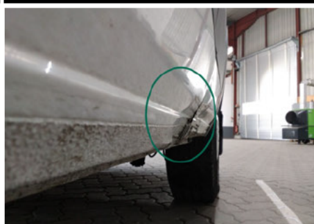
Schweller / Links / Delle
