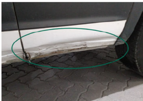
Schweller / Hinten Links / Delle
