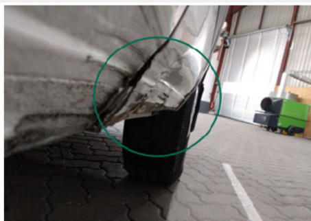
Schweller / Hinten Links / Delle
