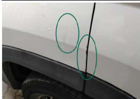
Kotflügel / Vorne Links / Delle
