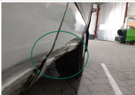
Schweller / Hinten Links / Delle
