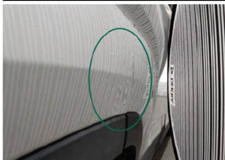
Kotflügel / Vorne Links / Delle
