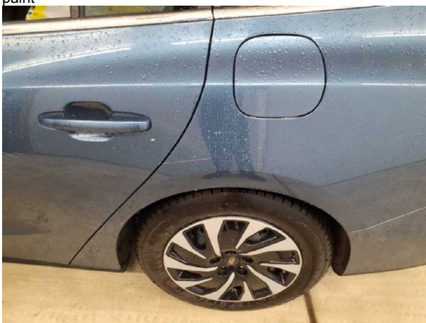
Damage #6: Side panel - rear left side: Side panel - Scratched - Repair and paint
