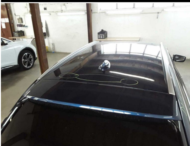
Damage #8: Roof: Roof - Deformed - Repair and paint
