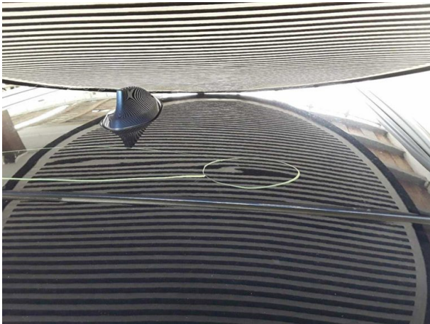
Damage #8: Roof: Roof - Deformed - Repair and paint
