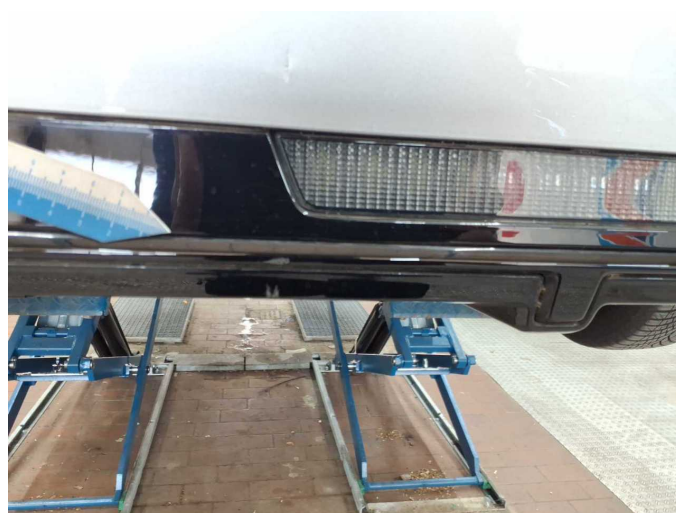
Damage 2: Rear bumper: Spoiler - Scratch(es) - Smart repair
