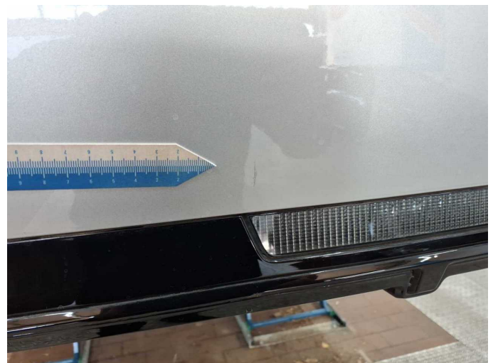
Damage 3: Rear bumper: Rear bumper - Scratch(es) - Paint
