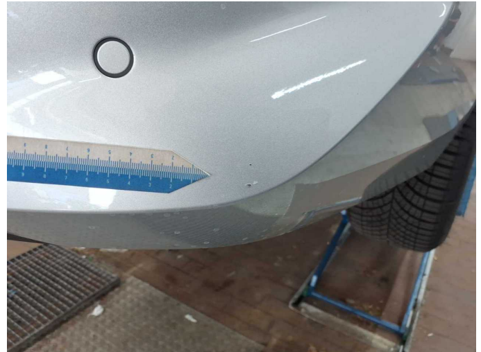
Damage 3: Rear bumper: Rear bumper - Scratch(es) - Paint
