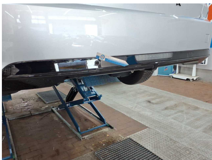
Damage 2: Rear bumper: Spoiler - Scratch(es) - Smart repair
