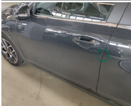
Tür / Vorne Links / Kratzer
