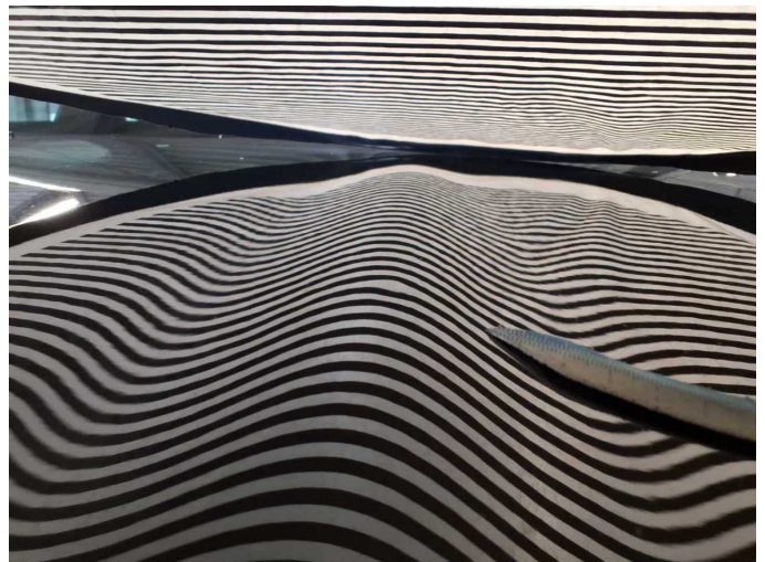
Damage 4: Bonnet: Bonnet - dent(s) - Smooth repair work
