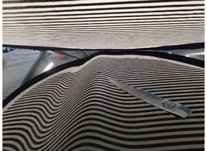
Damage 4: Bonnet: Bonnet - dent(s) - Smooth repair work
