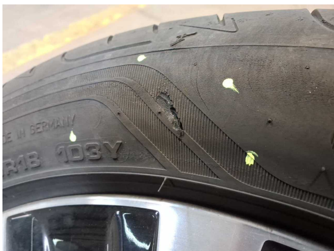
Damage 7: 2nd wheel set: 3 tyres (Flanke, lauffläche) - Damaged - Replace
