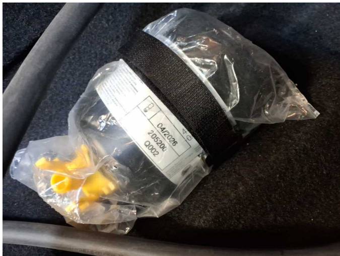
Damage 2: Equipment: Tirefit filler - Expired - Replace
