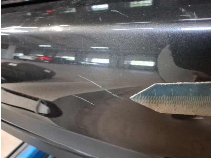
Damage 9: Rear bumper: Rear bumper - Scratched - Paint
