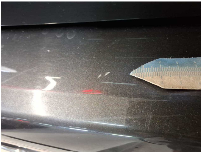
Damage 9: Rear bumper: Rear bumper - Scratched - Paint
