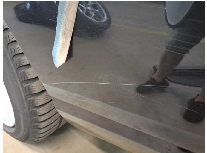
Damage 9: Rear bumper: Rear bumper - Scratched - Paint
