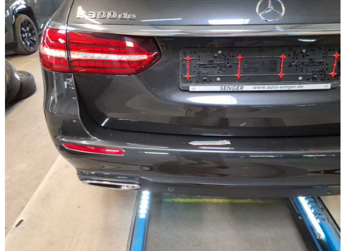
Damage 9: Rear bumper: Rear bumper - Scratched - Paint
