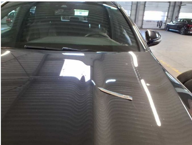
Damage 4: Bonnet: Bonnet - dent(s) - Smooth repair work
