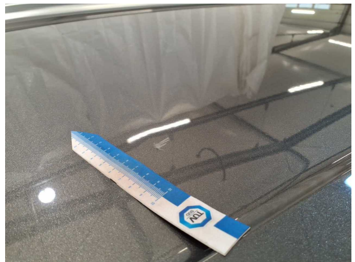
Damage 13: Roof: Roof - Dent / paintcoat damage - Repair and paint
