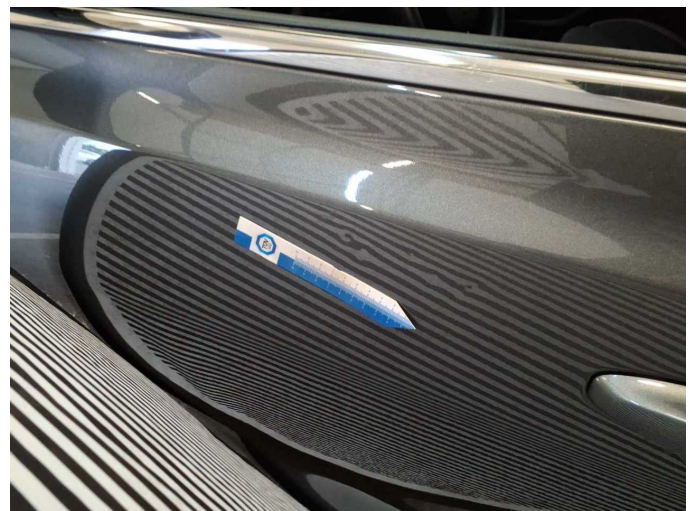
Damage 10: Door - front left side: Door - dent(s) - Smooth repair work
