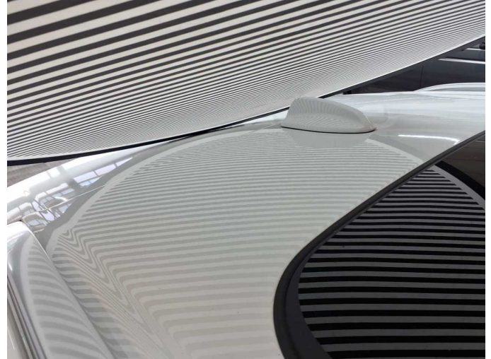
Damage 8: Body: Body - Damage by hail - repair according to calculation
