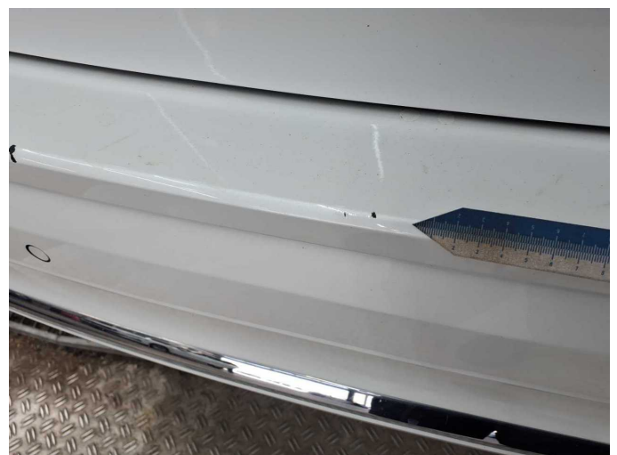
Damage 7: Rear bumper: Rear bumper - Scratch(es) - Paint
