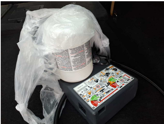
Damage 1: Equipment: Tirefit filler - Empty - Replace
