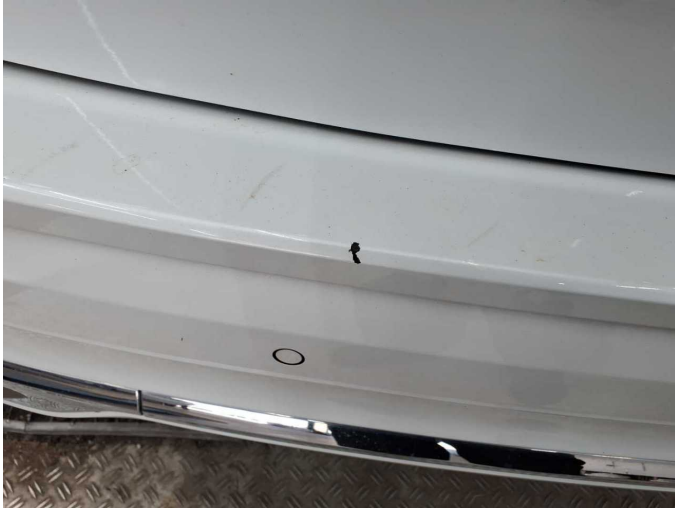
Damage 7: Rear bumper: Rear bumper - Scratch(es) - Paint
