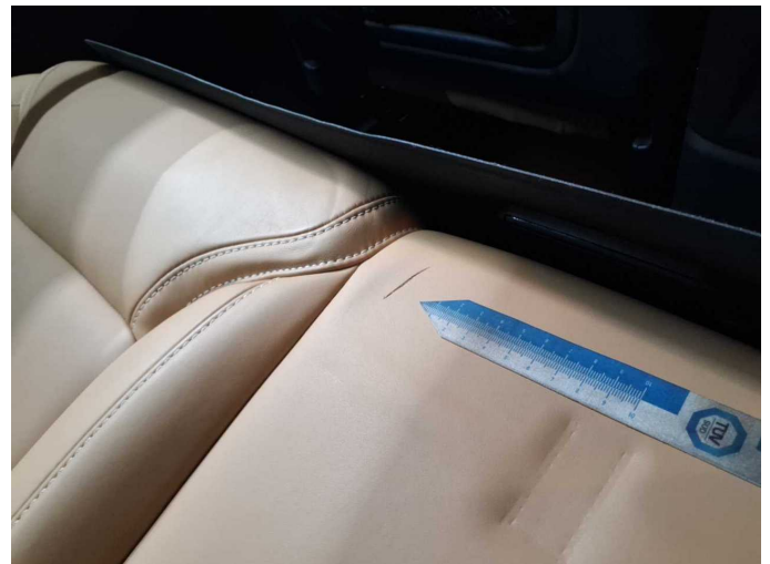
Damage 6: Seat - rear: Upholstery - Damaged - Replace
