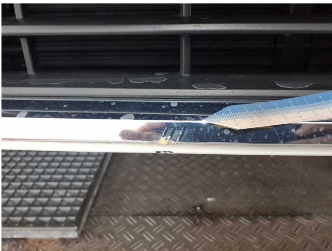
Damage 2: Front bumper: Protection strip - centre - Damaged - Replace
