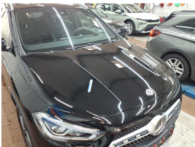
Damage 2: Bonnet: Bonnet - Stone chips - Paint
