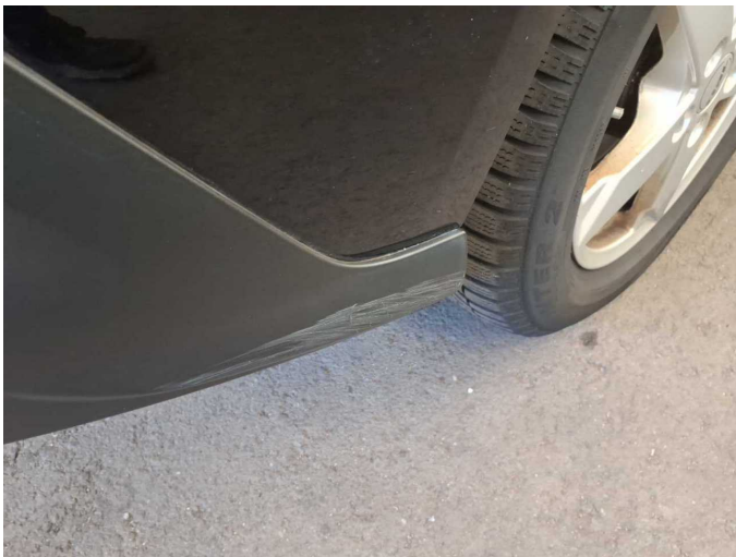
Damage 5: Rear bumper: Rear bumper - Damaged - Replace
