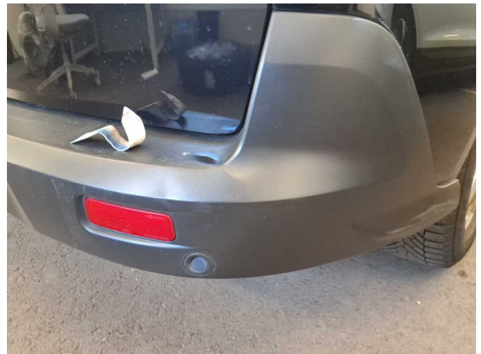
Damage 5: Rear bumper: Rear bumper - Damaged - Replace
