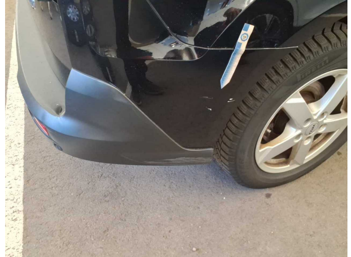
Damage 5: Rear bumper: Rear bumper - Damaged - Replace
