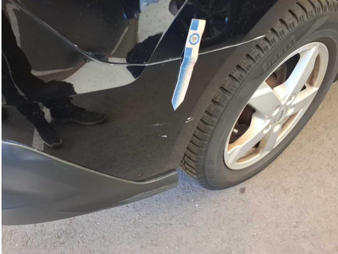
Damage 5: Rear bumper: Rear bumper - Damaged - Replace
