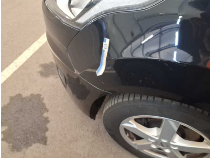
Damage 4: Mudguard - left side: Mudguard - left side - Scratch(es) - Smart repair
