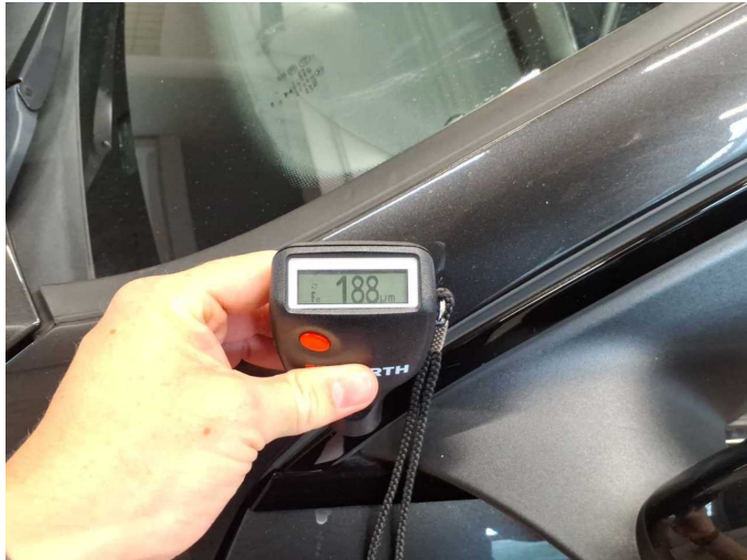
Repainting 2: Roof rail - left side
