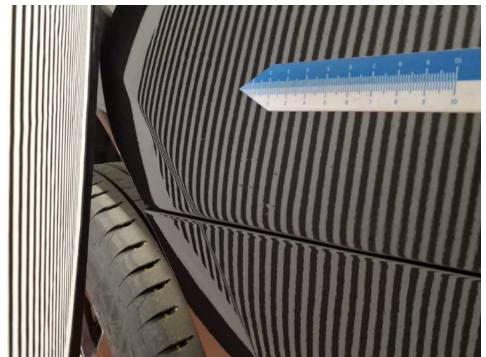
Damage 4: Side panel - rear left side: Side panel (Lackblasen) - Unprofessionally repaired - Repair and paint
