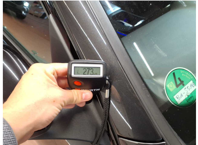
Repainting 3: Roof rail - right side
