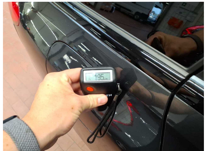
Repainting 5: Side panel - rear right side
