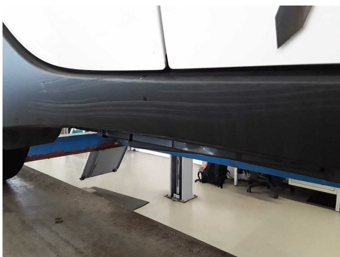
Damage 4: Sill - right side: Trim - Scratched - Replace
