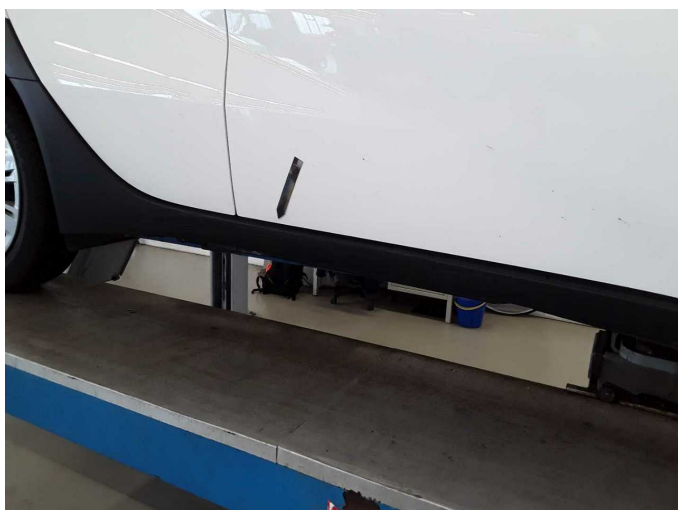
Damage 4: Sill - right side: Trim - Scratched - Replace
