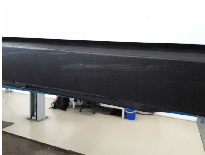
Damage 4: Sill - right side: Trim - Scratched - Replace
