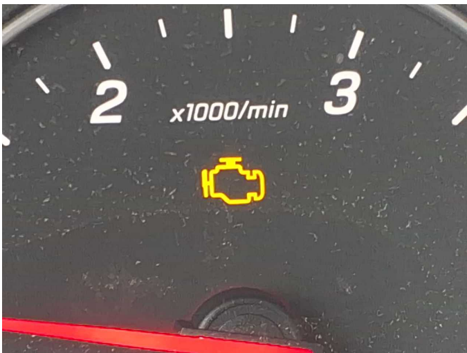
Damage 1: Instrument panel: Indicator light (Motorkontrollleuchte) - on - Perform diagnosis
