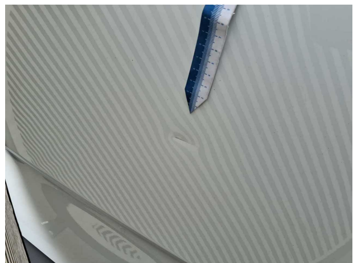
Damage 2: Boot lid / rear door: Rear door - right side - Dent / paintcoat damage - Paint
