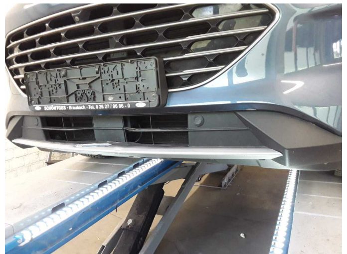
Damage 8: Front bumper: Spoiler - Deformed - Replace
