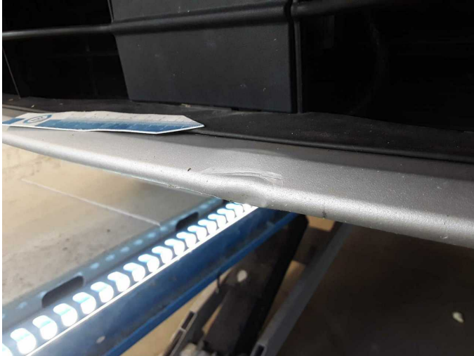
Damage 8: Front bumper: Spoiler - Deformed - Replace
