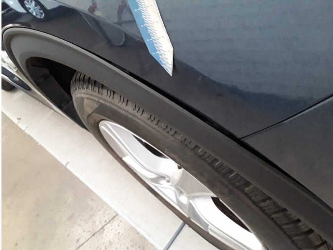
Damage 4: Mudguard - right side: Wheel arch - Play - Un- / install
