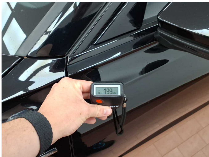
Repainting 6: Door - front left side
