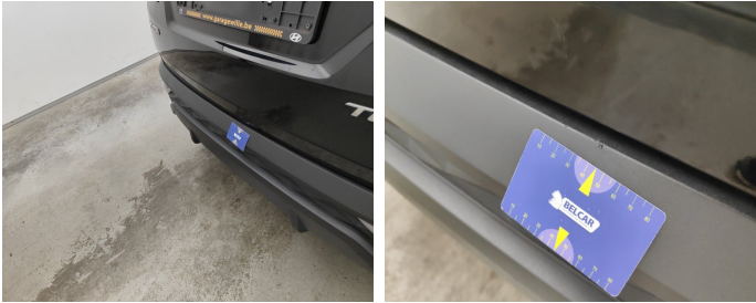
Bumper Rear / Lower Cover Not Painted / Replace-scratch
