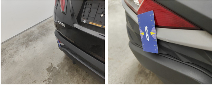
Bumper Rear / Trim Left / Replace-scratch
