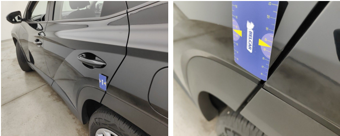
Door Rear Left // Smart Repair Small-scratch
