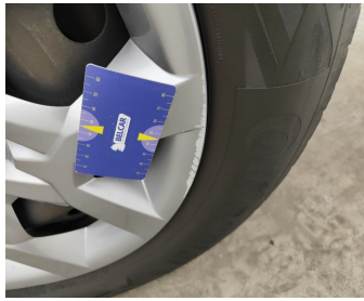
Wheel Alloy Front Right // Replace-scratch
