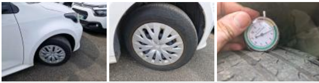
Tyre FL, Out of tolerance, Replace
