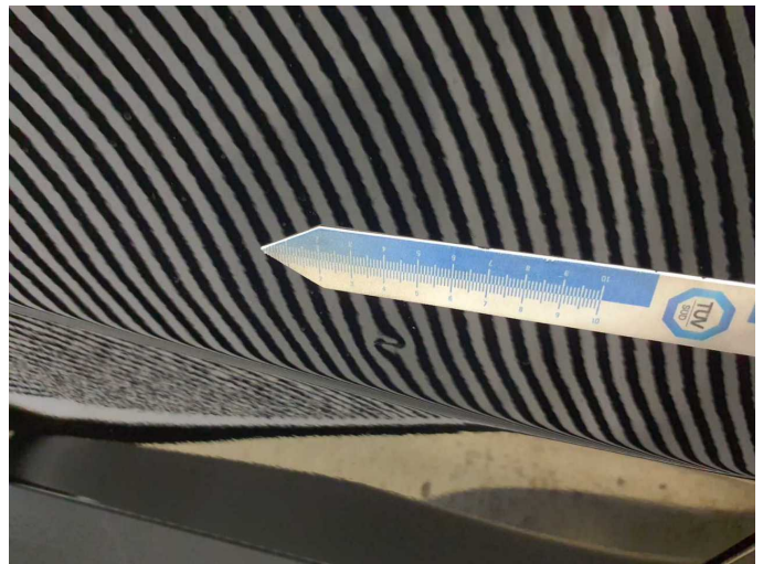
Damage 12: Door - rear right side: Door - Dent / paintcoat damage - Repair and paint
