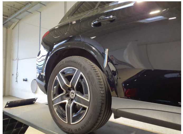
Damage 4: Side panel - rear right side: Wheel well extension - Scratch(es) - Paint
